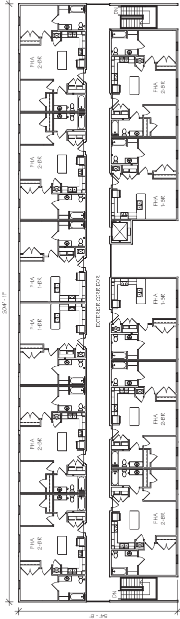
BUILDING #1 - 4TH FLOOR BUILDING PLAN
